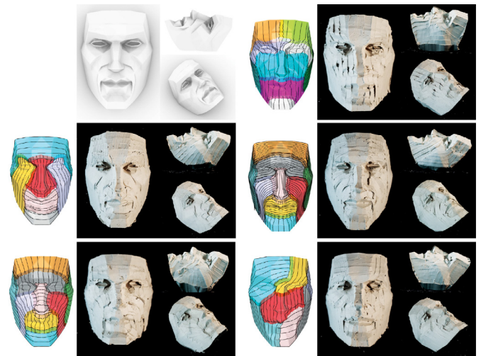
Fig. 16. Sculpting results of the face model. Top-left: input geometry; Rest: initial-ized toolpaths and the results with different styles by executing robot trajectories generated from our system.
