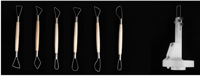
Fig. 3. Left: different manual loop tools used by professional sculptors; Right: our customized loop tool that can be attached to a UR5 as the robot end effector.
