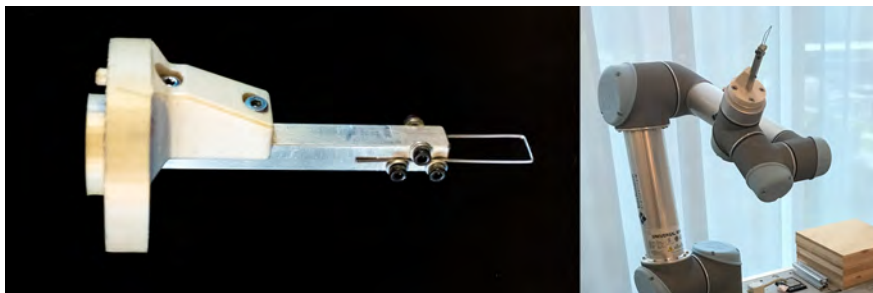
FIGURE 5.4: The customized loop tool and the UR5 with the tool attached.
