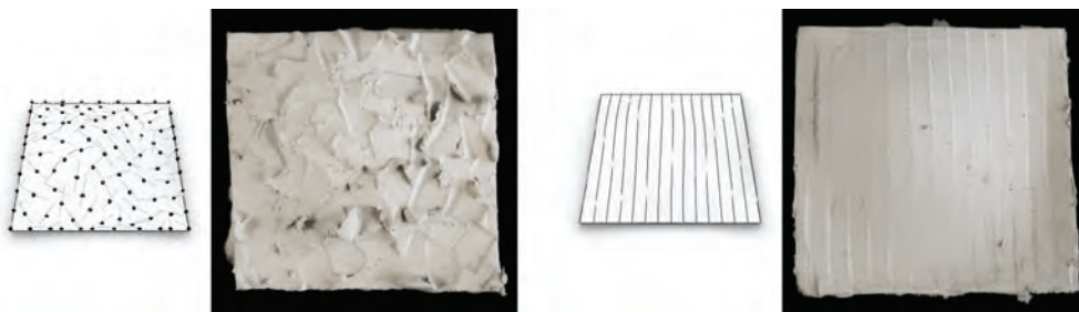
FIGURE 5.7: Point Sampling Sculpting Test. Left: a surface sculpted with 100 toolpaths of 18 mm length in random direction, generated from 100 randomly sampled points; Right: the same surface sculpted with 15 parallel toolpaths across the whole width of the patch.
