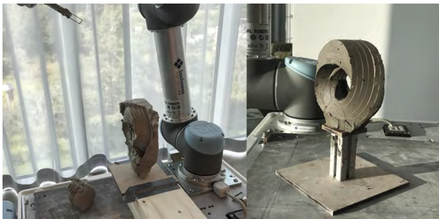
FIGURE A.6: The proof-of-concept model fabricated with the turntable prototype.
