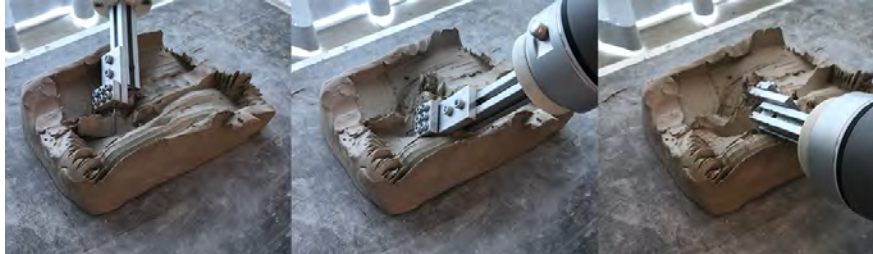
FIGURE A.3: Tool-target collisions observed in various sculpting paths.
