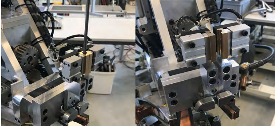
FIGURE 4.9: The new sleeve guide in its open and closed states.
