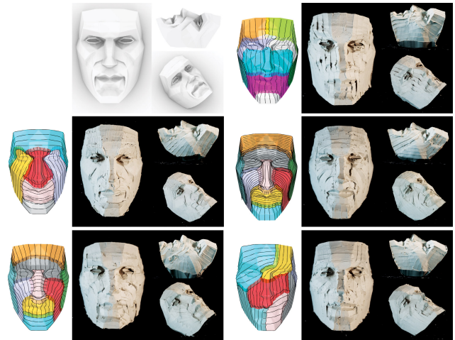
Figure 16: Sculpting results of the face model. Top-left: input geometry; Rest: initialized toolpaths and the results with different styles by executing robot trajectories generated from RobotSculptor .
