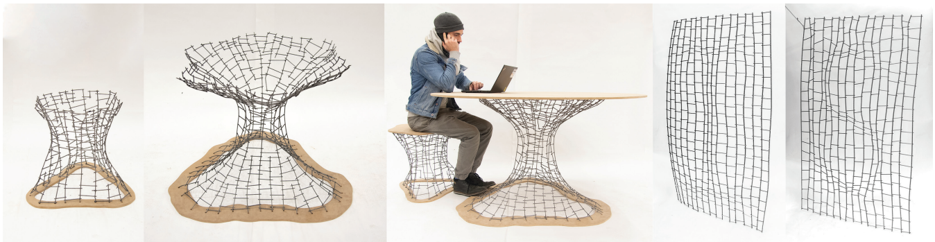
Figure 1: We present a computational method that aids with the design of structurally-sound metal frames, tailored for automated fabrication using existing robotic fabrication processes. By varying the density of bars, we enable transitions from narrower to wider regions (see chair and table designs, left), or the embedding of artistic targets (letters, right).
