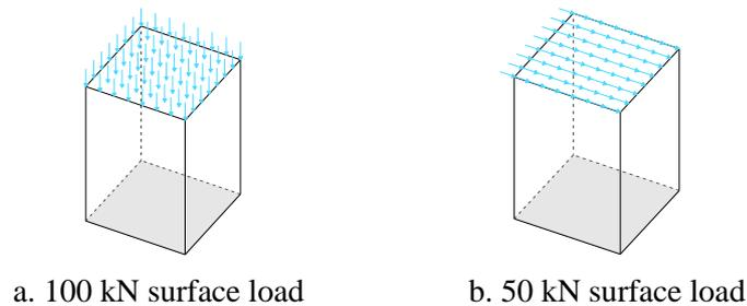
Figure 16: Two load cases for the testing geometry.
