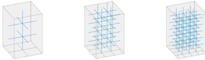
Figure 14: Testing volume filled with lattice of different density (base mesh 2x2, 3x3, 4,4)
